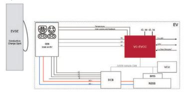
The EVCC is designed to be integrated into the vehicle with the following system architecture.
