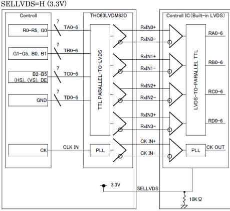
\*SELLVDS signal line has  $10 \text{ k} \Omega$  pulldown resister.
