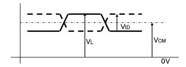
5)  $V_{CM}$ : LVDS Common mode voltage ( $V_{CM}$ =1.2V)
