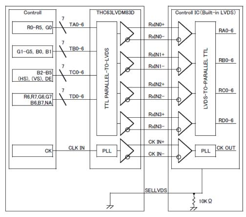
\*SELLVDS and signal line has 10 k  $\Omega$  pull-down resistor.
