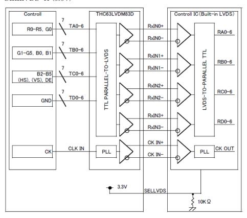
\*SELLVDS and signal line has 10 k  $\Omega$  pull-down resistor.
