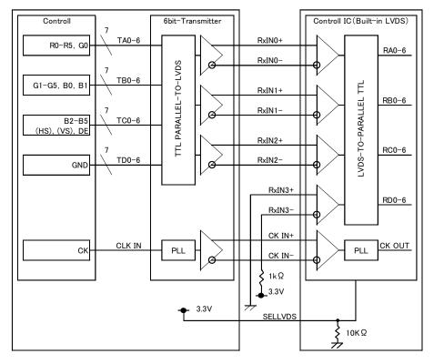
\*SELLVDS and signal line has 10 k  $\Omega$  pull-down resistor.
