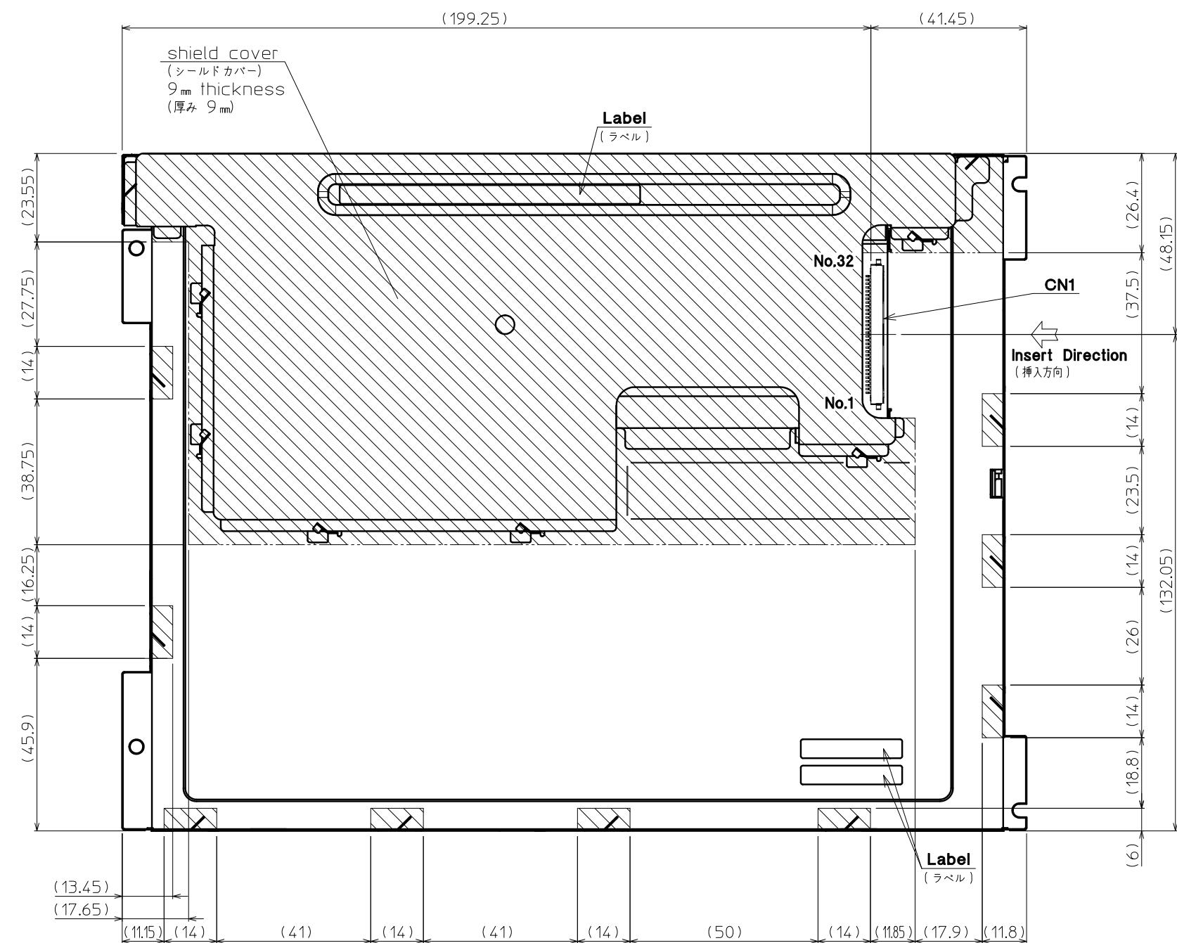
This drawing is a back side view of a flip horizontal to a front drawing.
