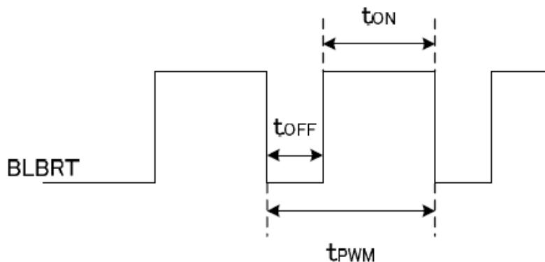
Please do not set **t<sub>OFF</sub>** with  $0 \mu\text{s} < t_{\text{OFF}} < 1 \mu\text{s}$ .
