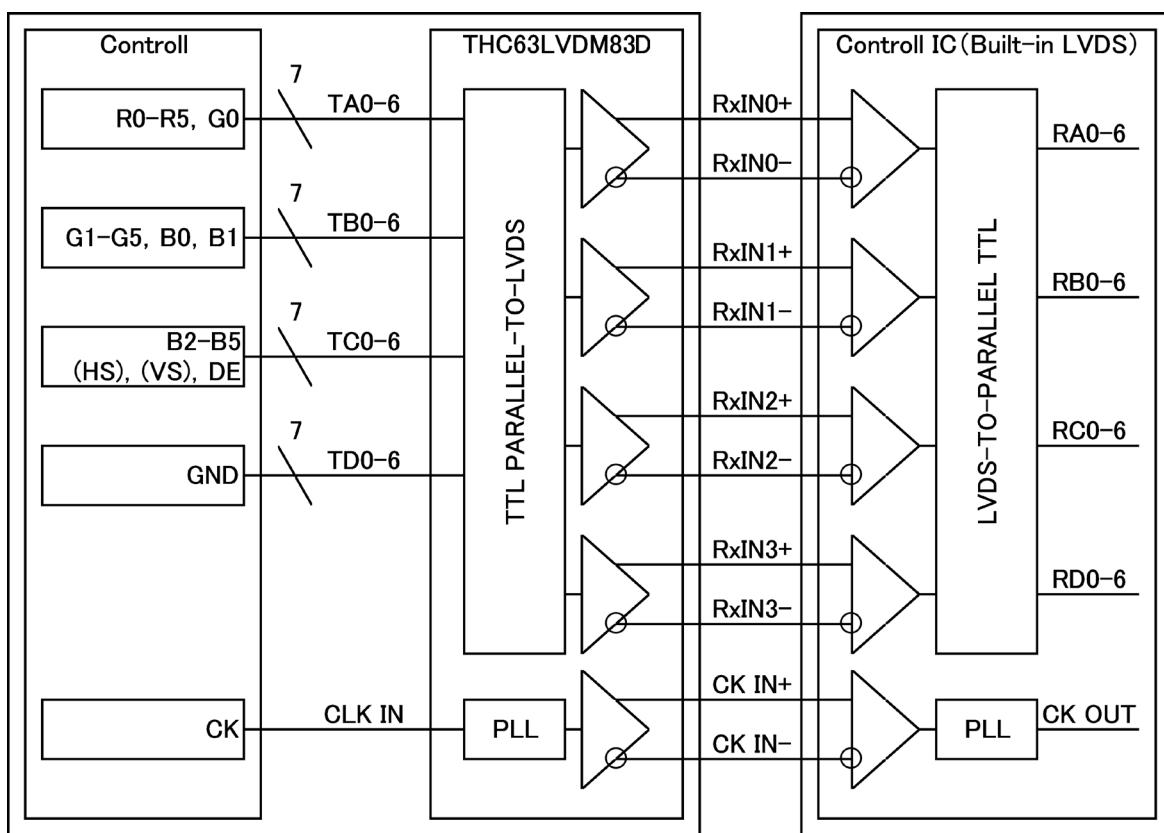
When using "6-bit Transmitter", please note that you are required to do the process of "surplus receiver" as following chart.
