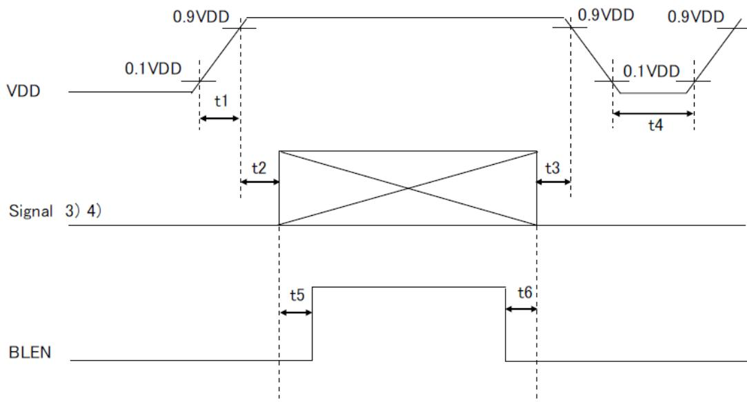
\* If the condition of t<sub>5</sub>, t<sub>6</sub> doesn't fill it, the display noise might be seen.
