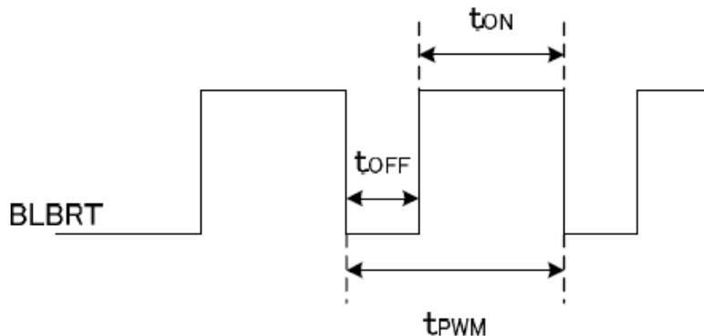
$t_{ON}, t_{OFF} \geq 50 \mu s$ .
