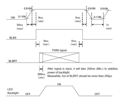
2)  $V_{IN} = 12V$ , Temp. = 25°C,  $D_{PWM} = 100\%$
