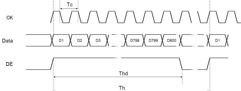
8-2. Input data signals and display position on the screen
