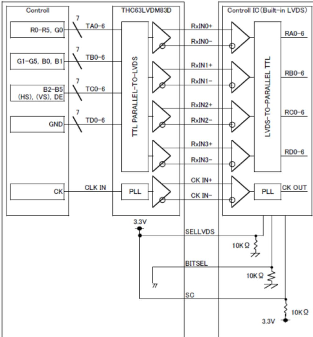
\*SELLVDS and BITSEL signal lines have 10 k Ω pull-down resistor.
