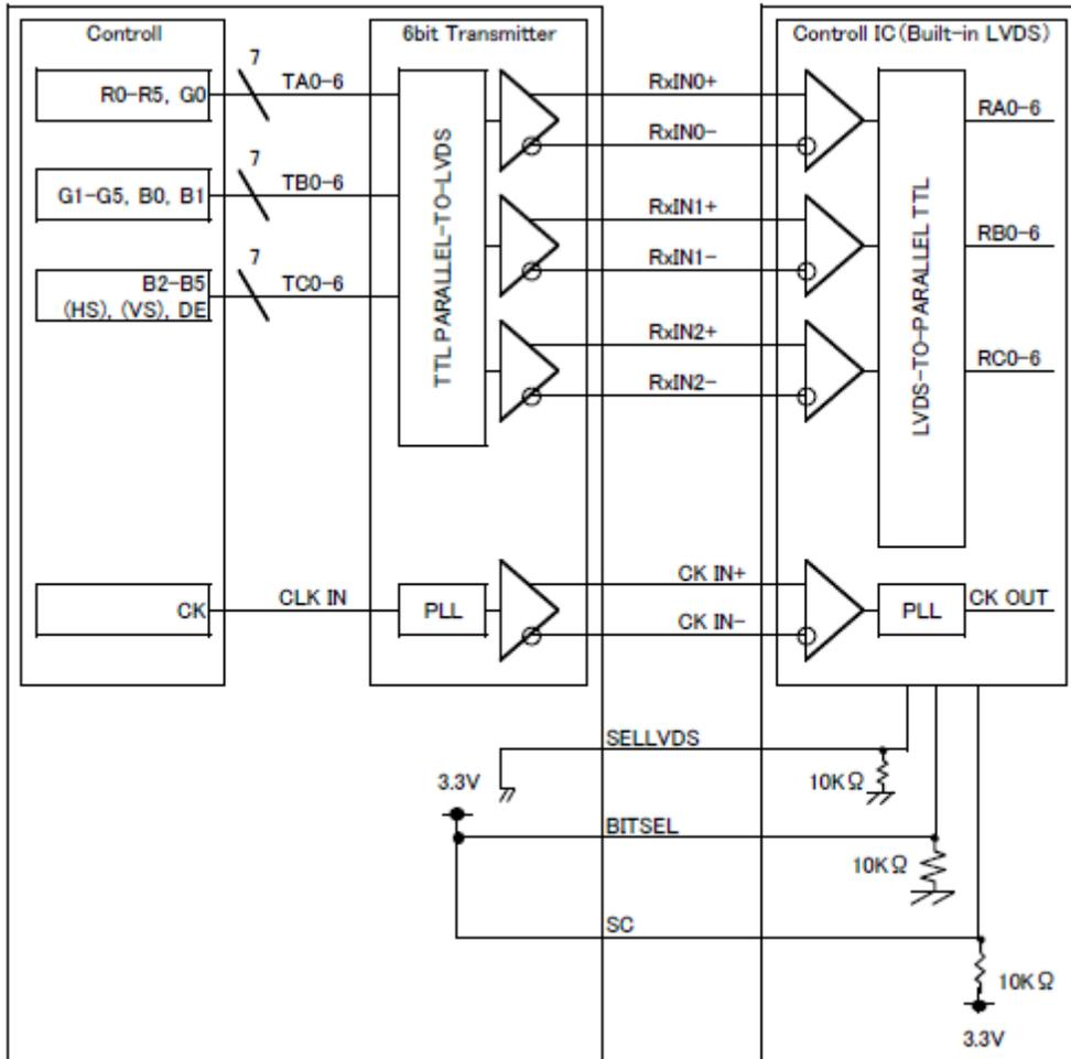
\*SELLVDS and BITSEL signal lines have 10 k Ω pull-down resistor.
