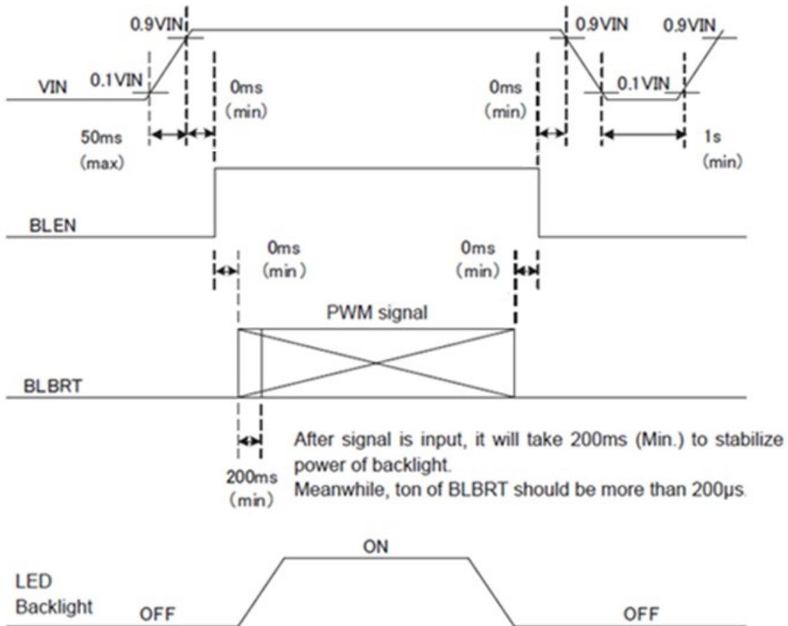
2)  $V_{IN} = 12V$ ,  $T_a = 25^\circ C$ ,  $D_{PWM} = 100\%$
