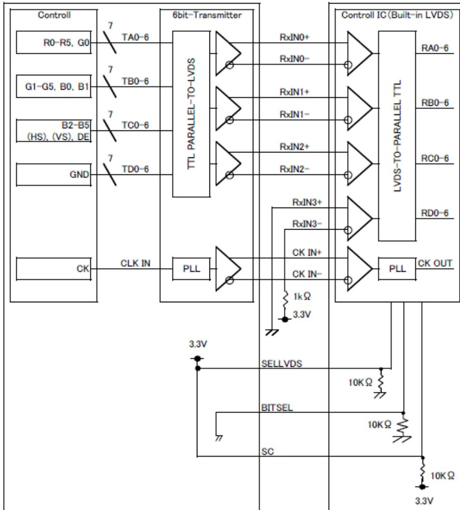
\*SELVDS and BITSEL signal lines have 10 k  $\Omega$  pull-down resistor.
