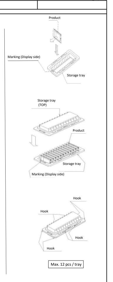
TCG057QVLCPANN\_Packaging Standard Packing pad 2. How to store LCDs in the box Storage tray Packing pad Packing pad Storage tray Packing pad Packing pad Outer Box (Corrugated cardboard) Max. 48pcs / outer box 3. Location of the labels PP band Confirmation label Shipping label 客先 品名 京セラ 株式会社 数量 検査者 検査者
