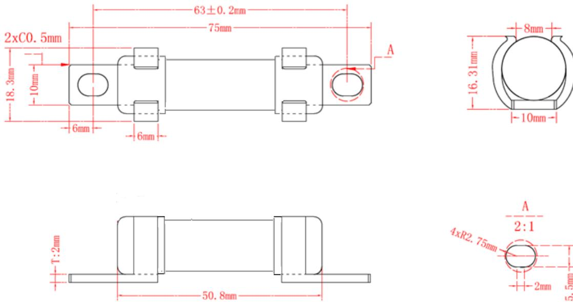
Note: recommend tighten torque: M5 – 4.5+/-1.0 Nm;
