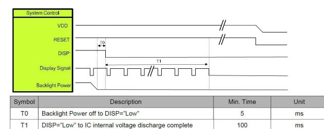
Note: When DISP pull "H" or "L", IC will execute the internal power on or power off procedures. Please be careful about the timing of DISP and do not interrupt it during power on or power off procedure, otherwise unexpected errors will occur.
