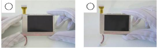
As above picture, please handle with anti-static gloves around LCM edges.
