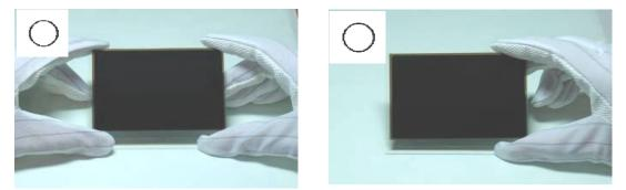
As above photo, please handle with anti-static gloves around LCD edges.
