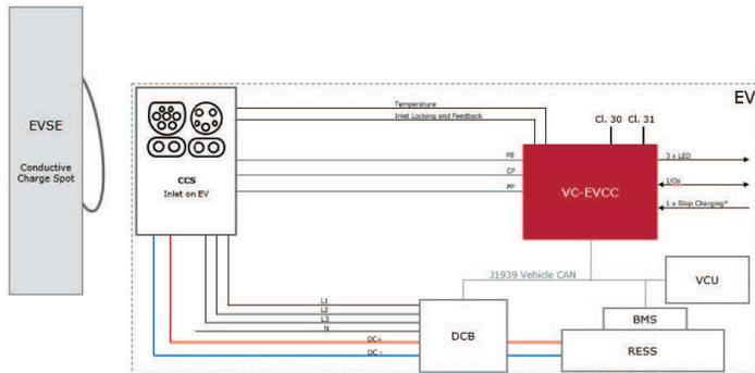
The EVCC is designed to be integrated into the vehicle with the following system architecture.
